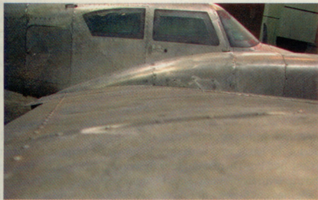
The airplane is continually cleaned throughout the paint process. Here's a view of the blasted skins after a Scotch-Brite cleaning. Though it's taken on a shine of sorts, we're still going to paint it.
