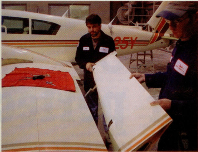
Control surfaces and fairings are removed prior to bead-blasting the old paint from the airframe.
